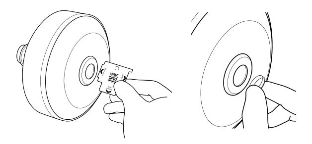
1 Remove the pre-assembled protective window by using the provided PTTOOL.
