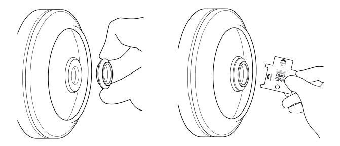
Screw PCCDLFAT in place using the provided PTTOOL.
